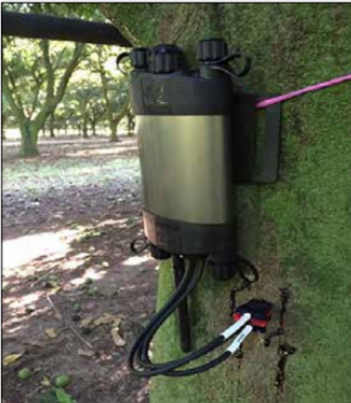
SFM1x Sap Flow Meter, ICT International https://ictinternational.com/products/sfm1/sfm1-sap-flow-meter/
