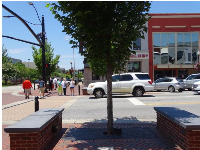
Permeable pavers allow water to reach tree roots. Tree at left is planted with sliva cell and above pavers that allow water through.
