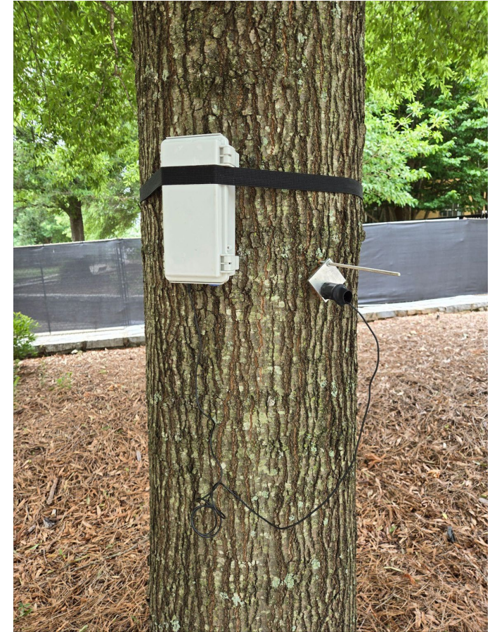
Dendrometer- data logger system attached to tree trunk
